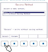
The **Saving Method** screen allows the user to save the modifications. To exit without saving, press scape or highlight *Exit Without Saving Method* option and then press scalect . To save the modifications highlight *Save Method* option and then press scalect .
