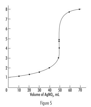
Figure 5 shows the titration of 50 mL of 0.1N NaCl with 0.1N AgNO<sub>3</sub>. The potentiometric signal is from a chloride ISE, and is plotted as pCl (-  $log [Cl^-]$ ).
