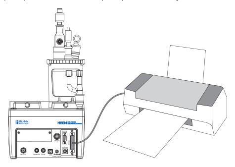
**Warning!** Connection/disconnection of POWER CORD, PUMP ASSEMBLY, PRINTER or BALANCE must only be done when titrator and external devices are turned off.
