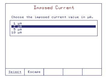
**Note:** Higher polarization currents will speed the contamination of the electrode and potentially degrade samples.
