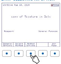
To select an option, press the option key below the virtual key. For example, to access the **Method Options** screen, press the option key below it.
