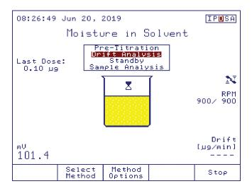
When the drift becomes stable the titrator switches to **Standby** mode.
