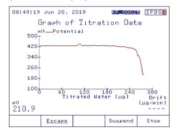
**Note:** For fresh solvents, the first few titration graphs may look a little noisy. After several titrations, the reaction speed and graph should improve.
