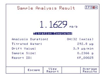
This screen displays information about the titration (duration, drift value used for compensation, sample size, titration report ID).
