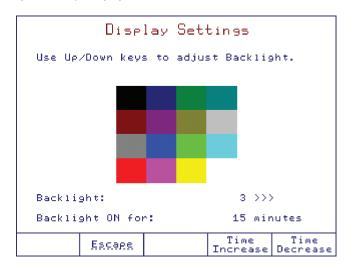
The displayed color palette allows for selection of appropriate backlight intensity.
