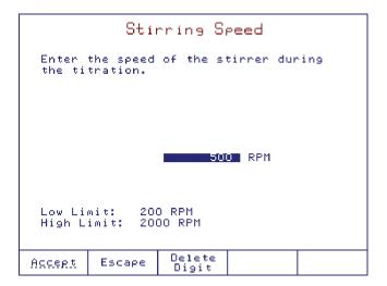
The stirrer will remain on for as long as the method is active. When the stirrer is running, the speed can be adjusted at any time by using the  $\wedge$  and  $\vee$  keys.
