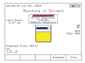
**Note:** If the pre-titration lasts longer than 30 minutes the titrator switches to **Idle** mode, errors may have occurred in your titration system (beaker is not properly sealed, wrong or missing regent, disconnected or faulty electrode, etc.). Check the system and start the pre-titration again.
