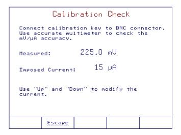
The electrode mV input and the electrode polarization current are measured with the **HI900941** calibration key and a  $mV/\mu A$  multimeter (not included).
