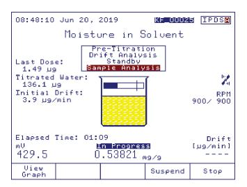
Press the stop key to stop the titration and return to **Idle** mode.
