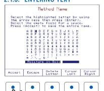
To enter text in an alphanumeric input box, first erase the previous text by using Delete Letter.
