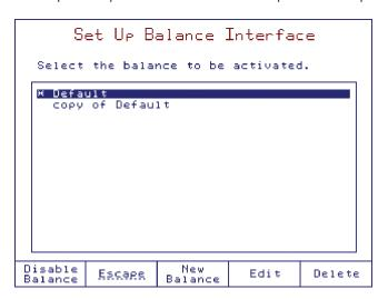
The balance is connected to the titrator via RS 232 interface.
