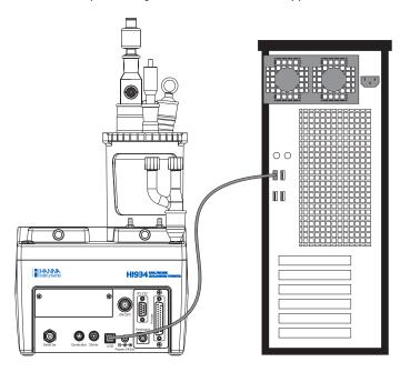
Connect the cable to the USB port on the rear panel of the titrator.
