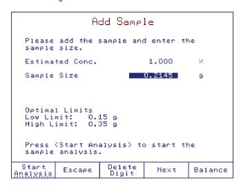
If necessary, update the estimated concentration. This value is used to determine the pre-titration volume. The optimal limits will be updated based on this value.
