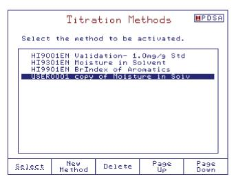
**Note:** The titrator can hold 100 methods (standard and user defined). When the limit is reached, a warning message is displayed.
