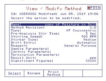
To exit the **View / Modify Method** screen, press the screen, and highlight *Save Method*. Press scleet to save modifications.
